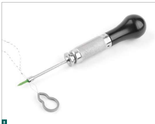
Fig. 8: Thanks to the slits in the screwdriver blade, the anchor screw can be screwed in with the thread inserted.
